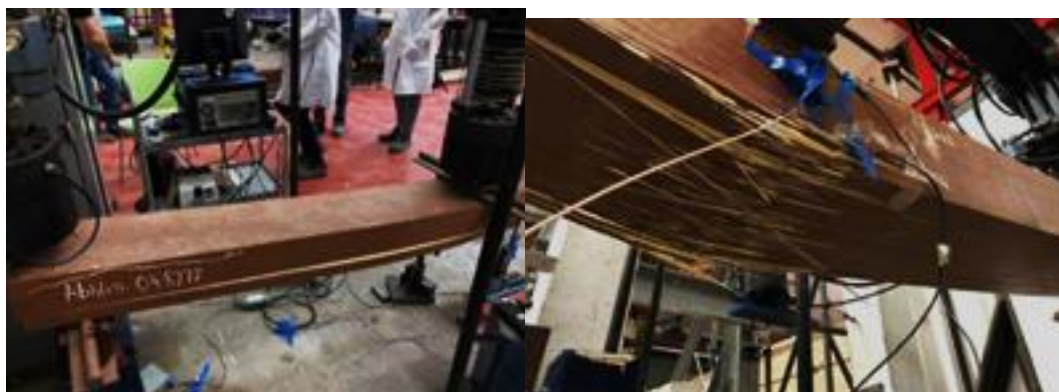
Fig. 7: Laboratory test showing failure mode (brittleness) of FFU composite bearers
