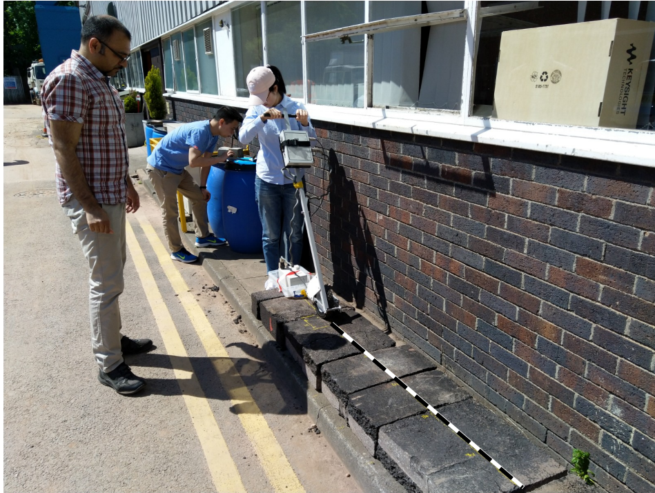
Figure 3: GPR unit traversing the cracked asphalt specimens
