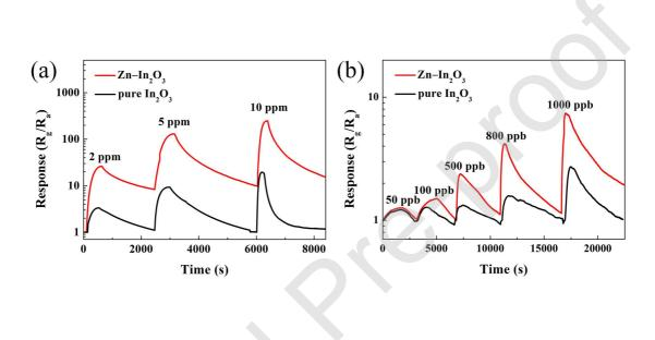
Fig. 7. Response–time curves of the sensors based on pure In<sub>2</sub>O<sub>3</sub> and Zn–In<sub>2</sub>O<sub>3</sub> nanofibers to various NO<sub>2</sub> concentrations at 50 °C: (a) 2–10 ppm and (b) 50–1000
