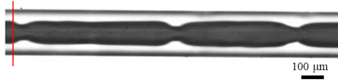
Figure 4 The position where the interfaces between fluid 1 and 2 is identified.
