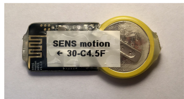
Fig. 1 Image of internal components of an accelerometer device – thigh worn SENS Motion Plus device, which measures 20 mm × 50 mm × 3.5 mm. Reproduced with kind permission of SENS Innovation
