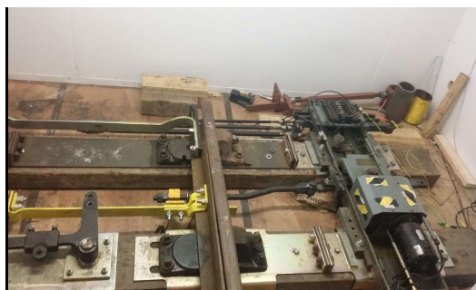
Fig. 3 The electro-mechanical switch actuating system located at the Birmingham Centre for Railway Research and Education (BCRRE), University of Birmingham (left); and the schematic diagram of a conventional switching layout (right): 1. stock rails, 2. switch rails, 3. stretcher bars, 4. common crossing, 5. check rails, 6. front-toe, 7. point operating equipment (POE), 8. actuator.
