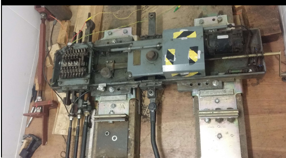
Fig. 4 The real electro-mechanical switch system (left); and its simplified schematic diagram.
