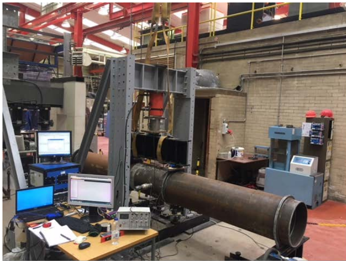
Figure 3: Schematic illustration of AE DAQ system (The AE sensors do not indicate the exact position during the tests)
