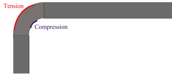
Figure 1. Simple schematic of a sheet undergoing bending, to illustrate tensile and compressive stress locations.
