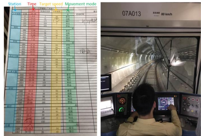
Fig. 6. Designed driver instruction material (left). Field test on Guangzhou Metro Line No.7 (right).
