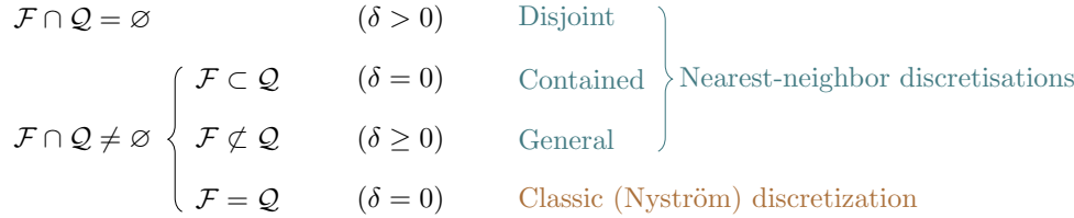
FIG. 1. Schematic detailing of the characterizations for potential force ( \mathcal{F} ) and quadrature ( \mathcal{Q} ) discretization sets with \delta , denoting the minimum distance between the discretizations, defined in (2.1). Each choice is further shown as belonging to either the set of nearest-neighbor or classic (Nyström) discretizations.
