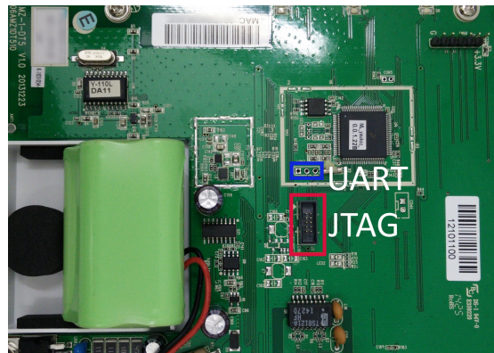
Fig. 2. Yale Easy Fit central unit PCB with UART and JTAG
