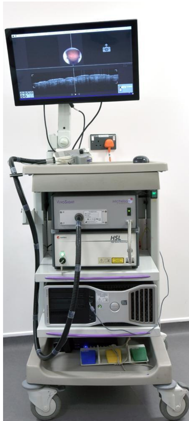
Figure 3. Swept-source optical coherence tomography scanner (Michelson Diagnostics VivoSight Rx). Copyright © 2017 Guy's & St Thomas' Hospital Trust: reproduced with permission.
