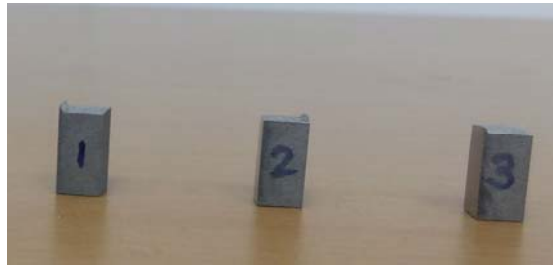
Fig 9. SLM coupons fabricated using the optimized process parameters
