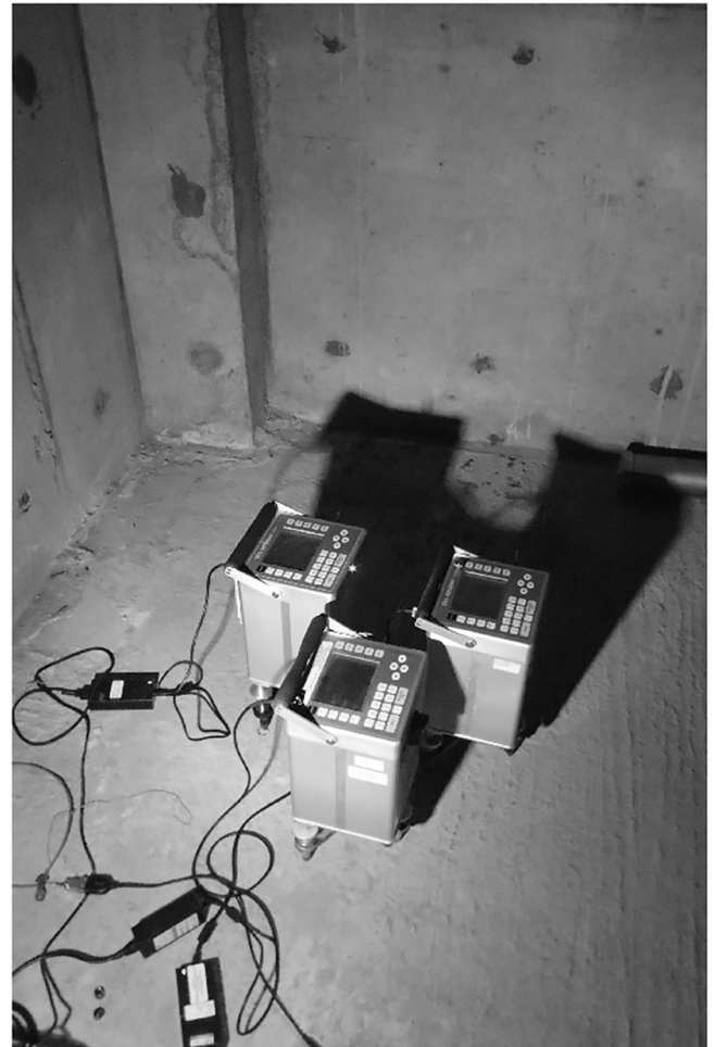
Fig. 2. The three instruments used to characterise the noise in the basement in the University of Birmingham.
