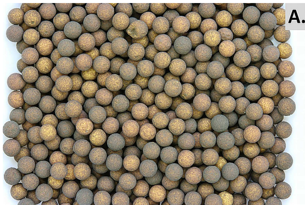
Figure 1: A - catalyst HiFUEL AB10 - pellets. B - External reformer (I) for planar cells (designed and manufactured by ALMUS AG).
