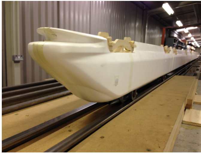
Figure 5: The TRAIN rig Class 373 Eurostar 7 car model.
