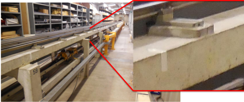
Figure 2: The concrete base of the testing rig.
