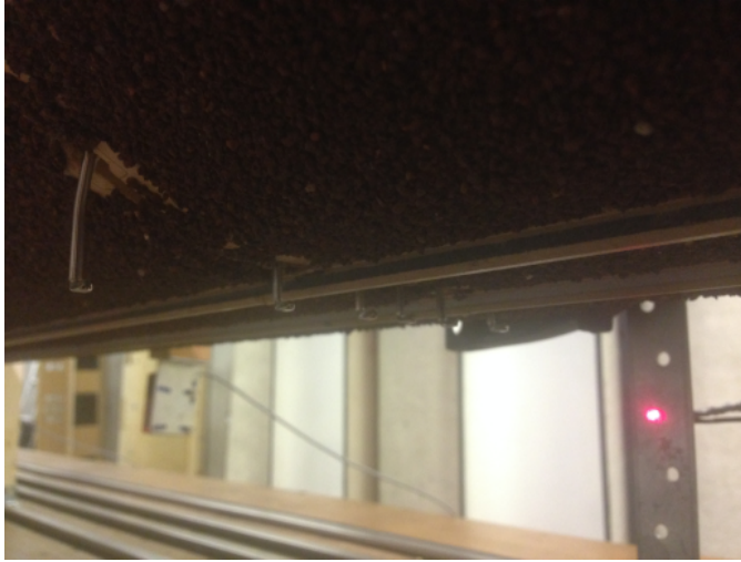
Figure 4: The multi-hole probe setup through the ground plane. The slit through which the instrumentation was placed is clearly visible, as is the simulated ballast roughness.
