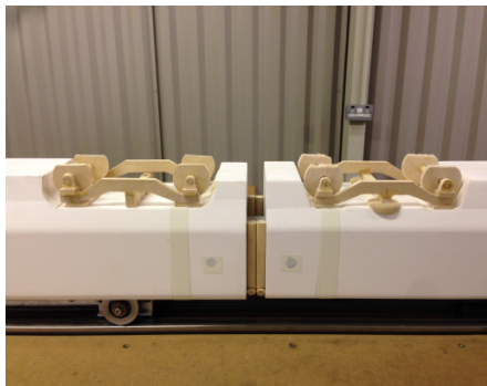
(a) Standard bogie inter-carriage region
