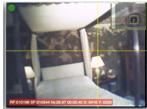
FIG. 4b. A frame from the rendered movie, combining the view from the participant's head with the view of their eye (inset top right). A calibrated model of the eye was fitted in Yarbus software. The cross hair in scene shows where the centre of gaze was directed.
