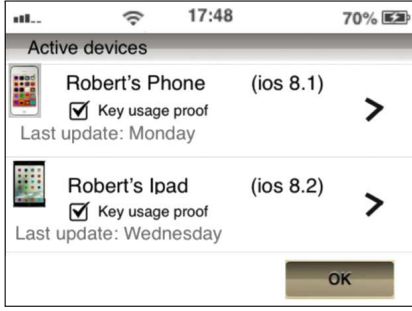
Fig. 3. An example of envisaged GUI that presents the table (D_i, t_i) for i = \{1, 2\} to Robert. The ticked box against the “key usage proof” indicates that the proofs about the usage statement (e.g., last update time) have been cryptographically verified.
