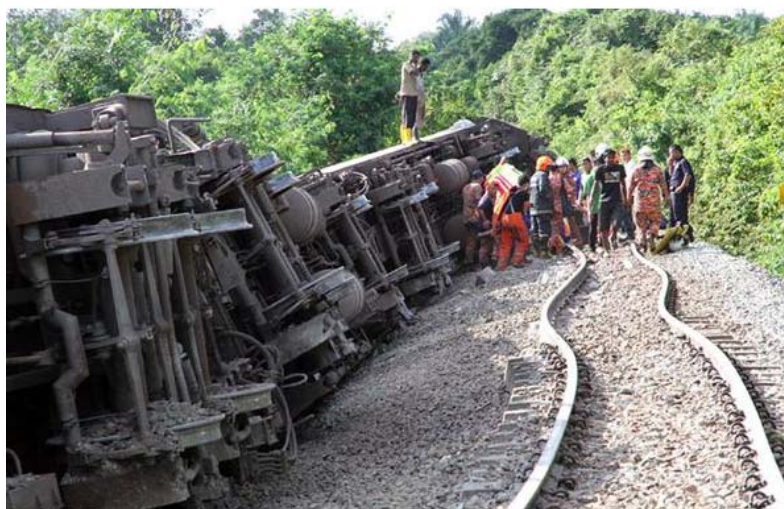
Figure 17. KTMB train derailed due to rail buckling and landed on its side, trapping the driver and injuring about five passengers just before Kempas, Johor station, southern part of Malaysia (Courtesy: Malaysia Department of Public Works).
