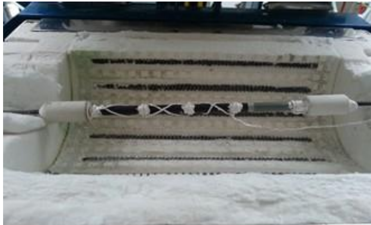
Figure 2: Tubular SOFC with manifolds.
