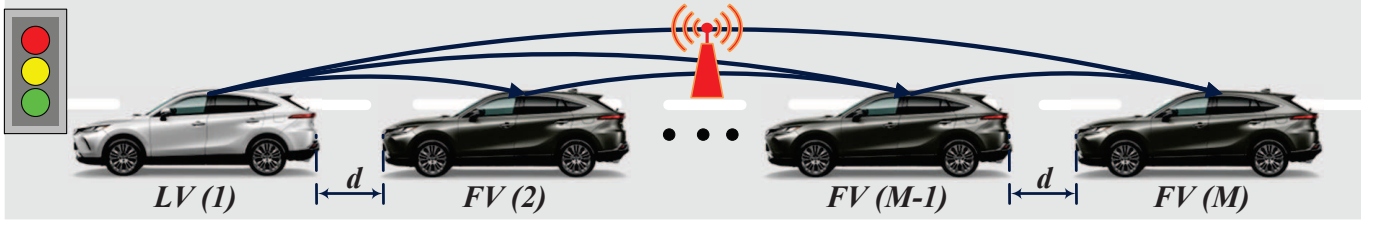
Fig. 1. Schematic diagram of vehicular platoon with PLF communication topology
