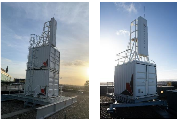
Fig. 2. Two L-band staring radars installed at UoB campus providing a testbed of networked radar to benchmark the MWP oscillator technology within a realistic urban environment.
