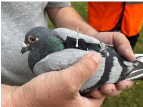
Figure 4 – Homing pigeon with a harness carrying a PathTrack GPS tag
