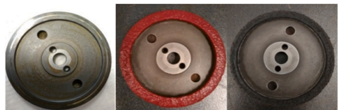
Fig. 1. Sample preparation of representative food soil, a: a plain MTM disc, b: fresh tomato purée placed on measurement area of the MTM disc, and c: burnt tomato purée after the thermal treatment.
