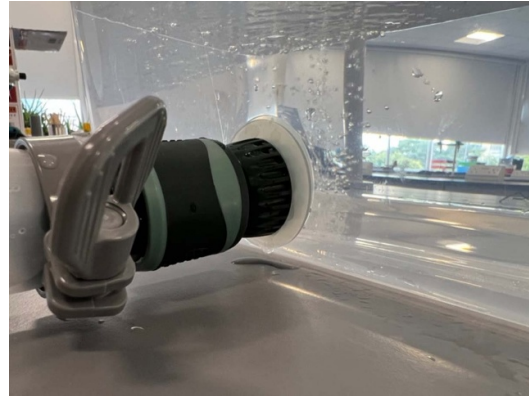
Figure 4. Hosepipe fitting used to connect pipe to the cold water bath.
