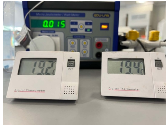
Figure 5. Digital thermometers and mains power meter used to obtain measurements.
