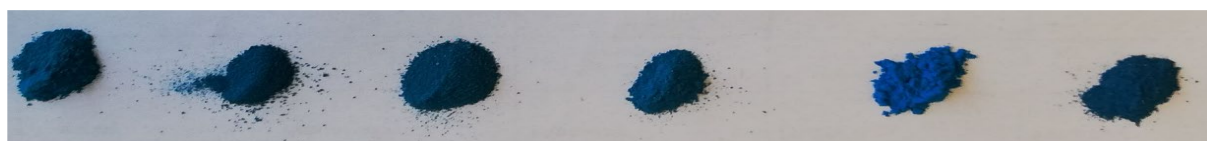
Figure 5: Colour image of \text{Ba}_{10-x}\text{Sr}_x(\text{MnO}_4)(\text{PO}_4)_5\text{Cl}_2 phases from left to right: x = 0, x = 1, x = 2, x = 3, x = 4 and x = 5
