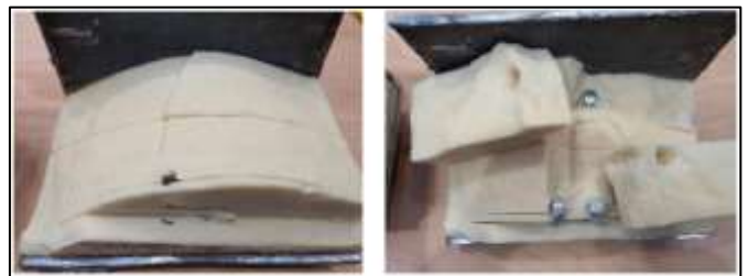
Figure 8: Cone failure line and hollo-bolt slippage of the FFT specimen
