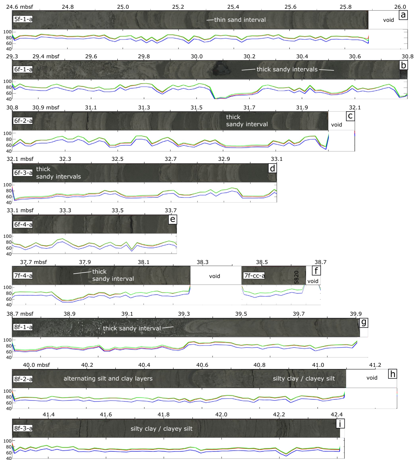
Figure 8. Line-scan images of sediment core at selected locations down core at Hole U1517C (see Figure 7 for depth intervals). Beneath each line scan are red-green-blue (RGB) values along scans. Depth labels on the tops of line-scan images are in meters below seafloor (mbsf), using the International Ocean Discovery Program Core Depth Below Seafloor B (CSF-B) scale. Some features in the core are annotated (see text for further descriptions).
