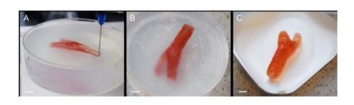
**Figure 3: Fabrication process of gellan carotid artery using SLAM.** (**A**) Extrusion of gellan within the fluid gel bed during printing, (**B**) completed carotid artery print within the fluid gel during crosslinking, and (**C**) final carotid artery model following retrieval from fluid gel support. Scale bars = 10 mm. Please click here to view a larger version of this figure.
