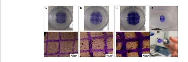
**Figure 1: Generation of high-resolution prints using SLAM.** Tailoring print resolution of alginate/collagen lattices as a function of filament diameter *via* extrusion at (**A**) 30 kPa, (**B**) 60 kPa, and (**C**) 120 kPa. (**D**) Generation of an alginate/collagen vascular tube. Scale bars = 400  $\mu$ m (**A-C**), 10 mm (**D**). Abbreviation: SLAM = suspended-layer additive manufacture. Please click here to view a larger version of this figure.
