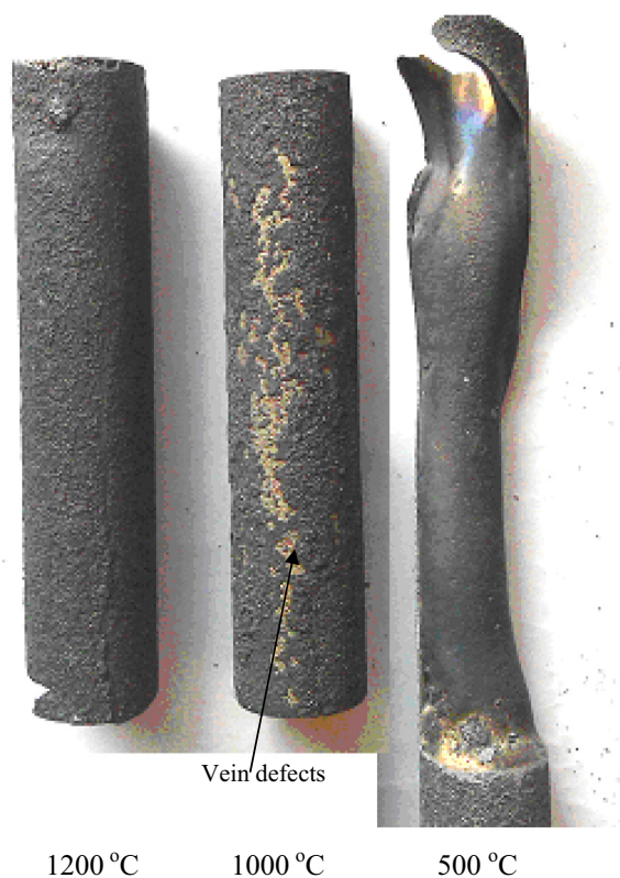
Fig. 4. The top part of cast bars of different mould pre-heat conditions.
