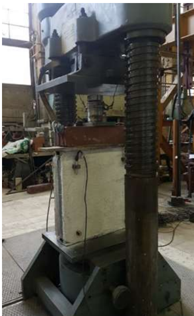
Figure 1a. Insulated composite wall specimen in 1:1 scale [5].
