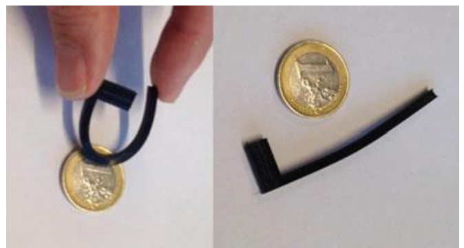
Fig. 27. 3D printed flexible antenna enabled by LM [178].
