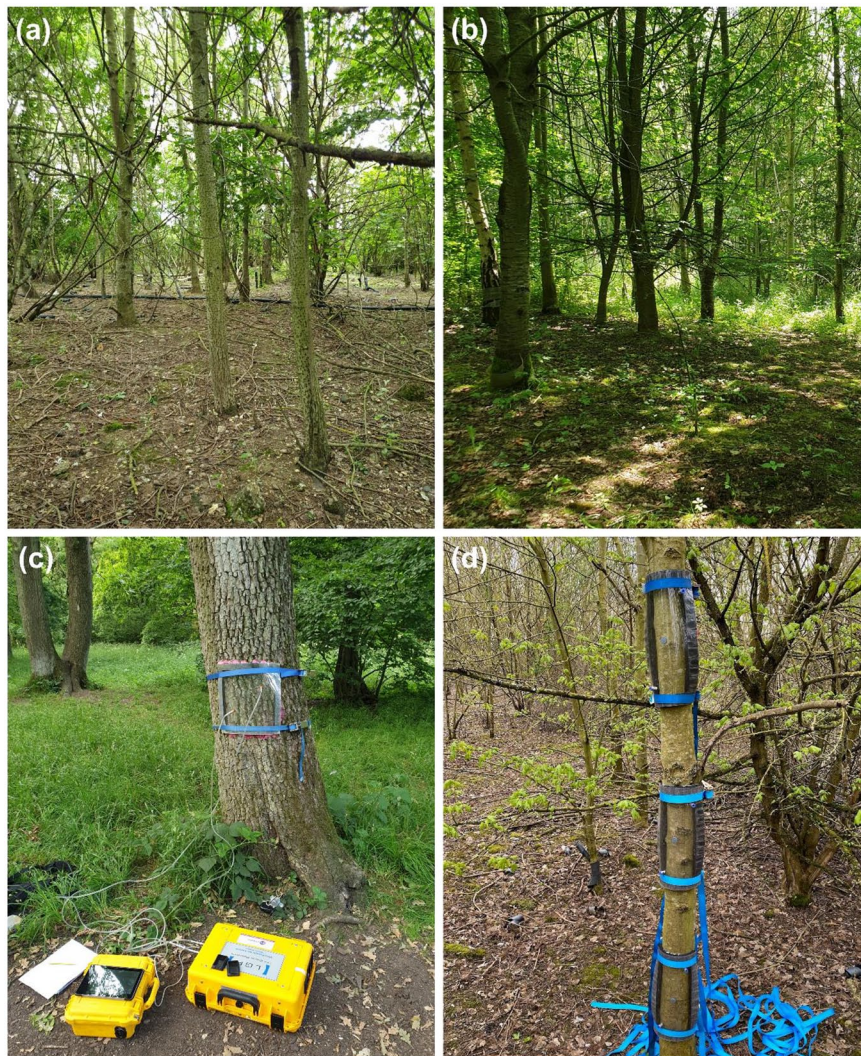
Figure 1. (a) The sampled landfill site, (b) the sampled non-landfill comparison site, (c) the gas sampling method which used a recirculating closed-loop system between gas flux chambers and a GHG analyser, and (d) gas flux chambers affixed to a tree.
