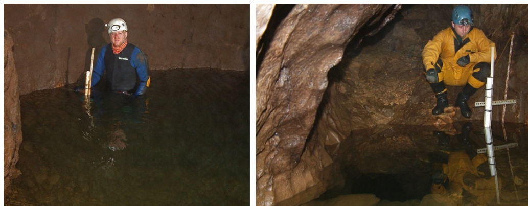
Figure 5. Stilling wells installed at Main Rising (left) and Whirlpool Rising (right).
