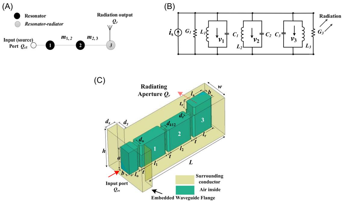
**FIGURE 1** Diagram of the proposed filtering antenna: (A) topology, (B) equivalent circuit, and (C) physical configuration. The resonators are coupled by the mutual capacitances. Dimensions in mm are  $a = 22.86$ ,  $b = 10.16$ ,  $t = 2$ ,  $t_r = 9$ ,  $l_o = 10$ ,  $d_0 = 6.0$ ,  $d_{k12} = 3.18$ ,  $d_r = 2.31$ ,  $l_1 = 26.0$ ,  $l_2 = 24.47$ ,  $l_r = 19.85$ ,  $l_a = 19.0$ ,  $h = 40$ ,  $w = 24$ ,  $L = 88$ .
