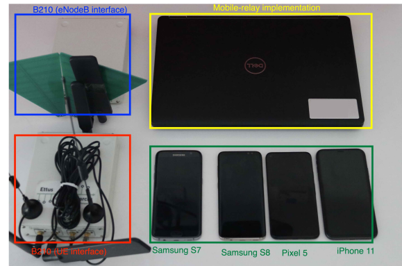
Figure 5: Experimental setup. Our mobile-relay software implementation runs on the laptop computer. Two USRP B210 SDRs are connected, one acting as an eNodeB and the other as a UE interface.
