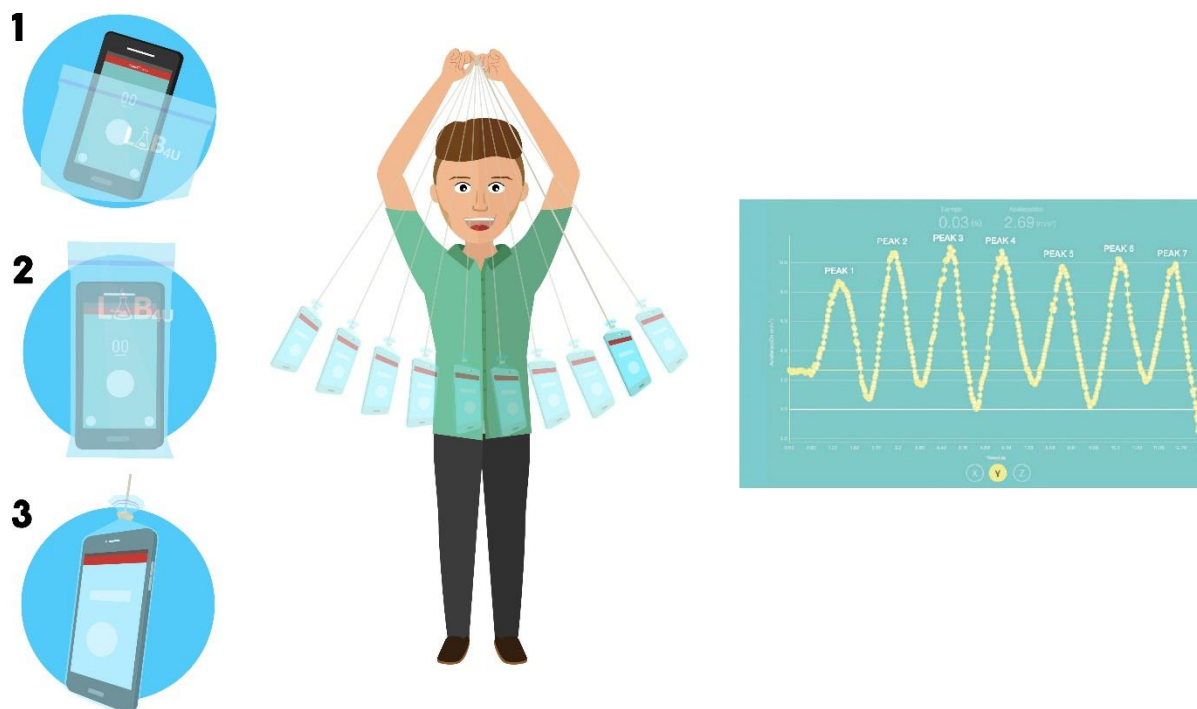
Figure 1. Screenshots of the Pirate Ship activity, showing how to set up the experiment (left), the procedure (center), and the graph that is obtained after conducting the activity (right).
