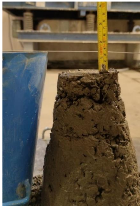
Figure 1. Slump test of the M_3 concrete mix.
