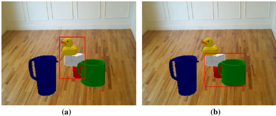
Fig. 6 Examples of ROIs automatically identified by the attention mechanism for further analysis in the context of estimating: (a) stability of object structures; and (b) occlusion of objects
