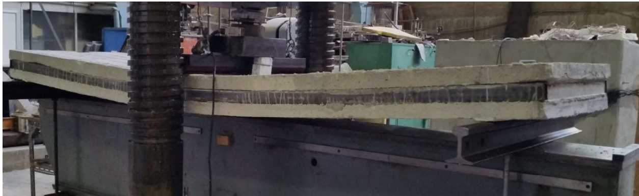
Figure 2. Out of plane bending test on the elementary module of double-shell composite wall
