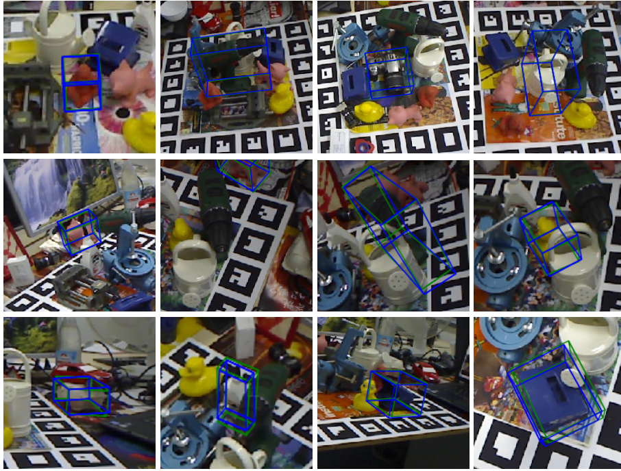
Fig.4. Qualitative pose estimation results on LINEMOD and Occlusion LINEMOD dataset. Green 3D bounding boxes denote ground truth. Blue 3D bounding boxes represent our results. Our results match ground truth well.
