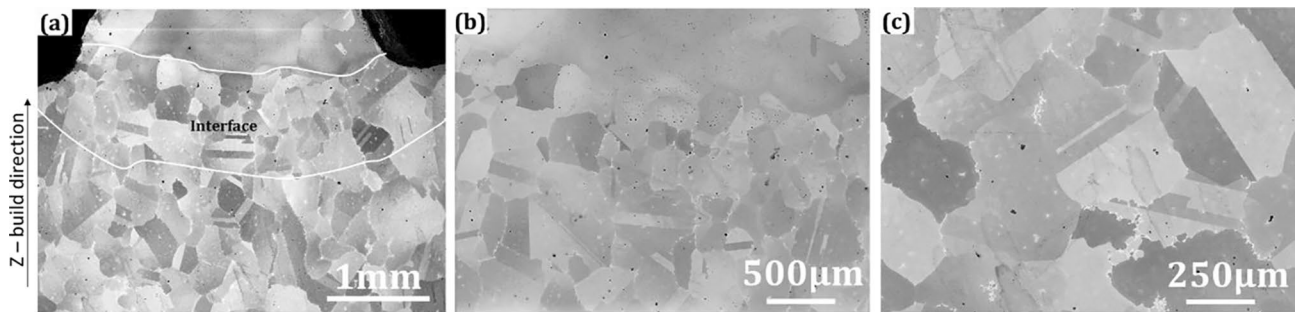
Fig. 9 Micrographs of the HT hybrid part: a the interface between the deposited structure and the substrate; b higher magnification image of the interface area; c the microstructure of the substrate
