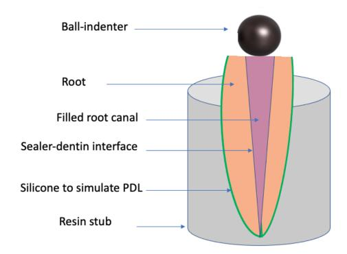
Figure 1S: Schematic diagram showing the experimental setup during fracture resistance study
