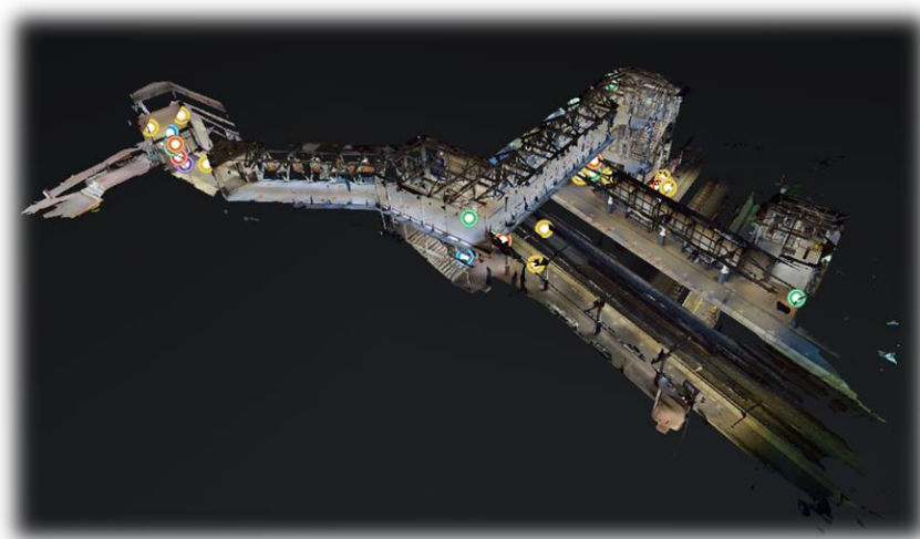
Figure 3: Dollhouse view of the point-cloud of Smethwick Galton Bridge (SGB) station.
