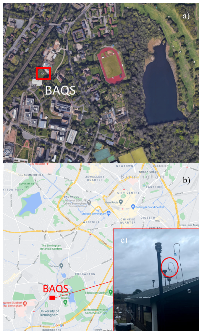
Figure 1. (a) Location of the Birmingham Air Quality Supersite (BAQS) (aerial view), (b) location of BAQS in relation to Birmingham, UK, and (c) sampling inlet used for low-cost sensors.
