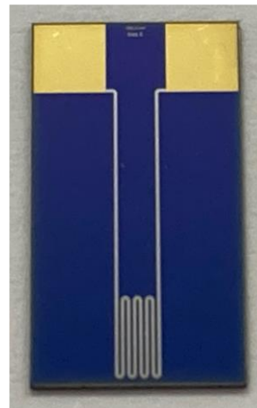
Fig. 8. Fabricated chip after being cut by the laser.
