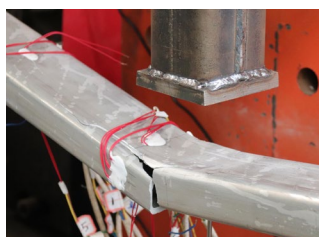
(a) Material tensile fracture (RTB100-50-W-A)
