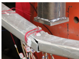
(a) Material tensile fracture (RTB100-50-W-A)
