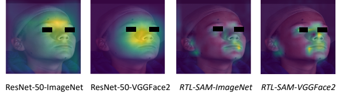
Fig. 9. Illustration of top activation attention maps for models with different pre-trained source tasks: the source model (ResNet-50) pre-trained on ImageNet (ResNet-50-ImageNet), the source model (ResNet-50) pre-trained on VGGFace2 (ResNet-50-VGGFace2), the proposed regularization constraint on spatial attention maps transferred from ImageNet pre-trained weights ( RTL-SAM-ImageNet ), and the proposed regularization constraint on spatial attention maps transferred from VGGFace2 pre-trained weights ( RTL-SAM-VGGFace2 ).
