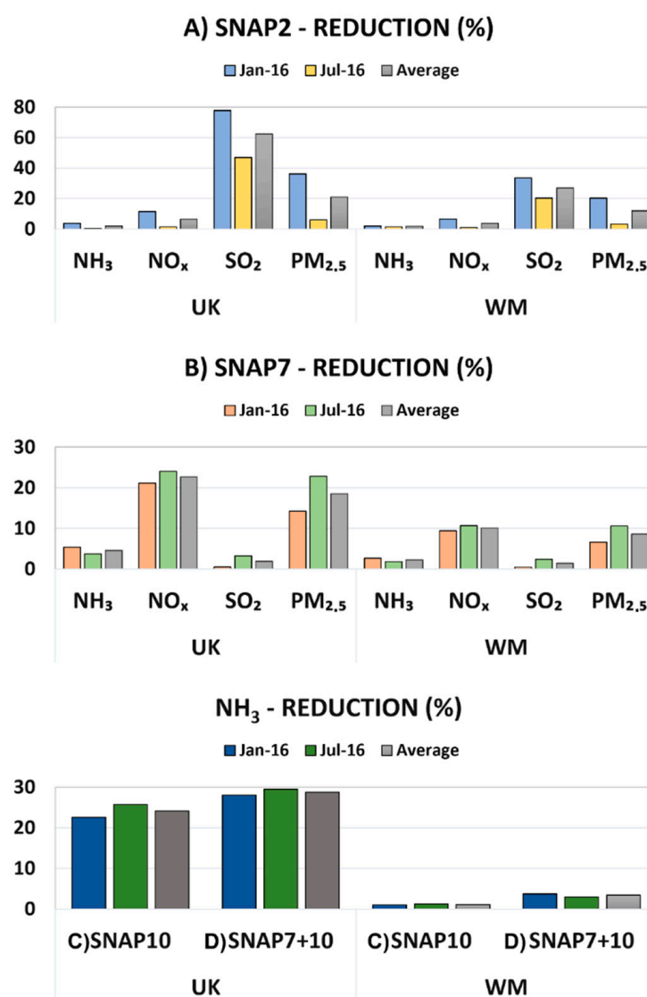
Figure 3. Percentage reduction of the total monthly emissions (January, July and average), across all sectors combined, for scenarios A (SNAP2, (top)) and B (SNAP7, (middle)), for NH 3 , NO x , SO 2 and primary PM 2.5 . The percentage reduction of NH 3 from scenarios C (SNAP10) and D (SNAP7+10) is shown on the (bottom) panel for January, July, and their average. The reductions are shown for the UK-wide reductions (UK) and for local reduction (WM) options.
