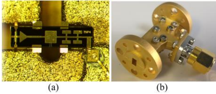
Fig. 4. Pictures of the fabricated frequency doubler: (a) the fabricated MMIC placed in the 3D-printed waveguide split-block; (b) the assembled doubler.
